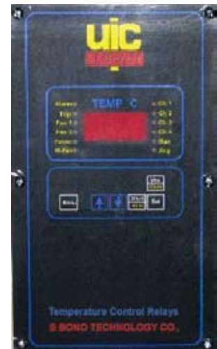
Temperature Indicator and Controller Power: 110/220V, 50/60Hz Contactor: AF Control, Alarm & Trip Temperature Range: 1°C~199°C Sensor: PT-100Ω x 3 Protocol(option): RS485/4~20mA
