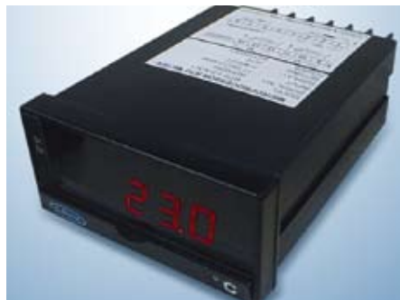
Temperature Indicator Power: 110/220V, 50/60Hz Contactor: Alarm & Trip Temperature Range: -100°C ~ 400°C Sensor: PT-100Ω Protocol(option): RS485/4 ~ 20mA
